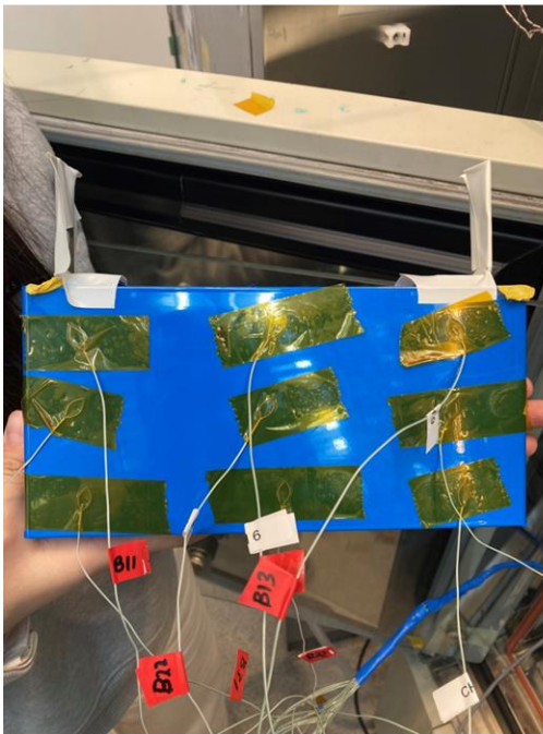
a. Thermocouples on the back side of the cell
