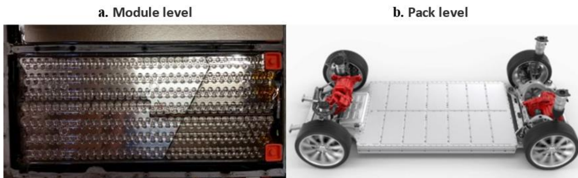
Figure 1.4 Battery of Tesla Model S: module level (a) and pack level (b) [18,21].
